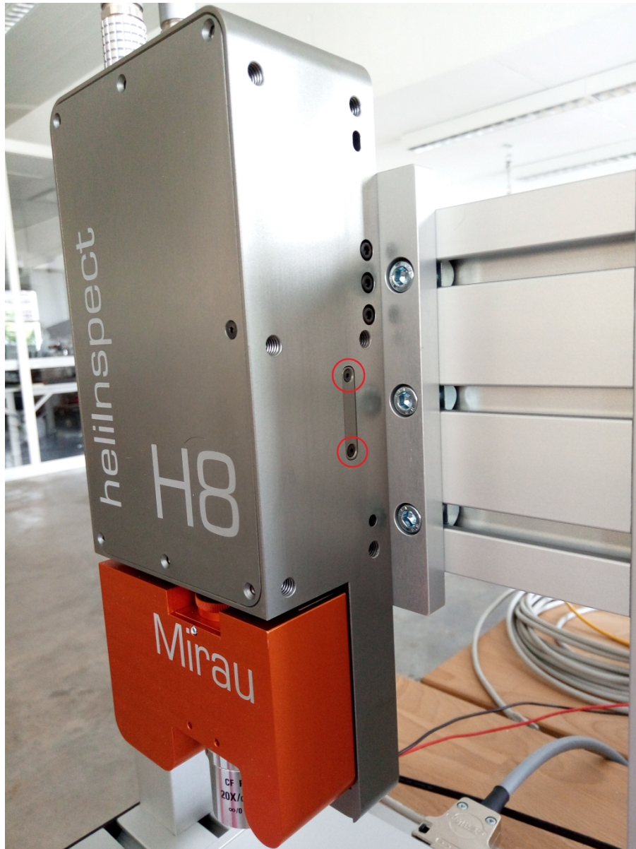
Fig. 1.2: SD-Card Cover Screws
